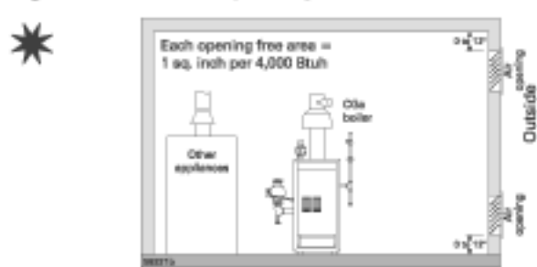
Figure 3 Air directly through outside wall
